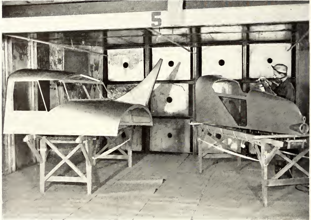
FIGURE 5-98.—Typical spray booth for finishing aircraft parts by spraying. The operator wears a mask for protection against paint mist.
